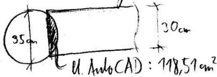
$$\sigma_{c,\frac{\alpha}{2},d} = \frac{N_d}{118,51 \text{ cm}^2} = 0,238 \frac{\text{N}}{\text{cm}^2} \hat{=} \underline{2,38 \frac{\text{N}}{\text{mm}^2}}$$
